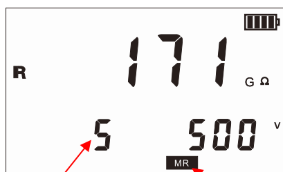
Figure 13-1 Resistance check
