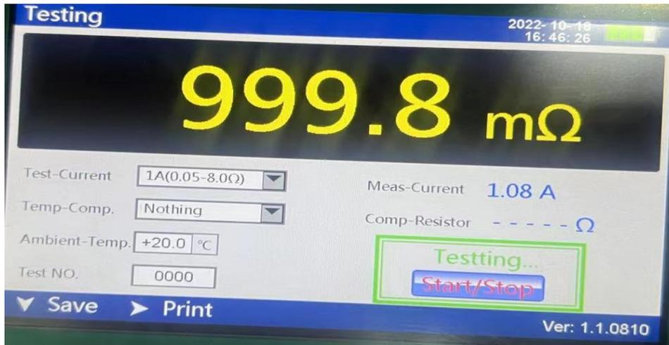
3. After the test, press the "stop" button, the instrument power off, LCD screen restore the initial state, rewire for the next measurement, or turn off the power supply and remove the test line and power cord to end the measurement.
