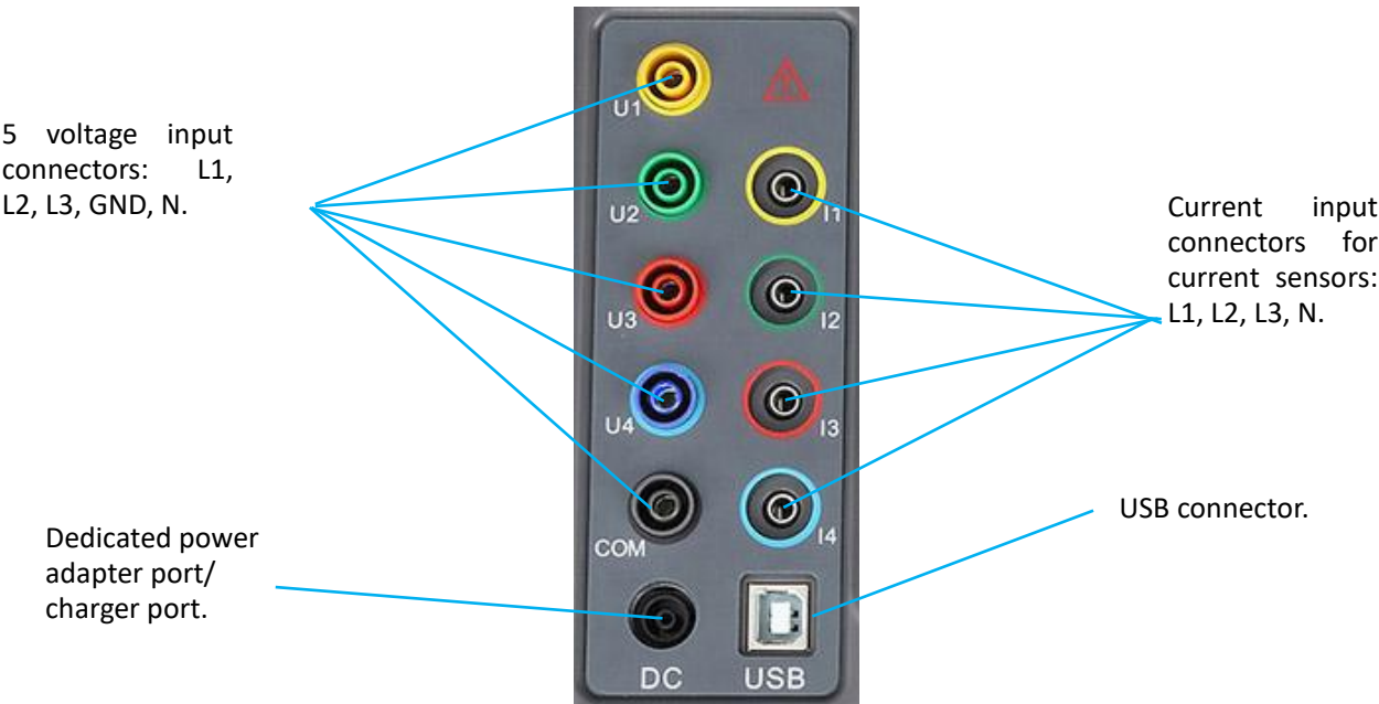
Figure 3-3: Connectors on the top of device
