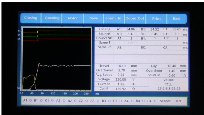
(2) **Opening test:** click this menu, opening voltage output, measuring opening time, three-phase different period, speed and other parameters.
