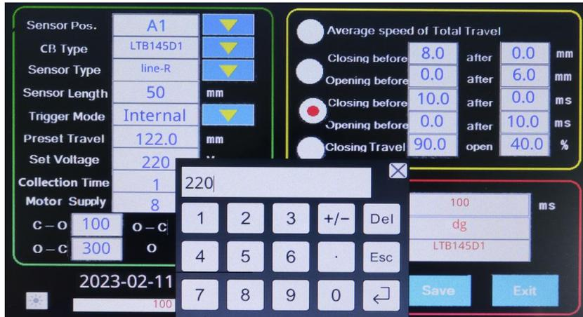
(8) **Acquisition time:** under normal circumstances, the acquisition time as long as 1 second can be, time can be set 1-10 seconds.
