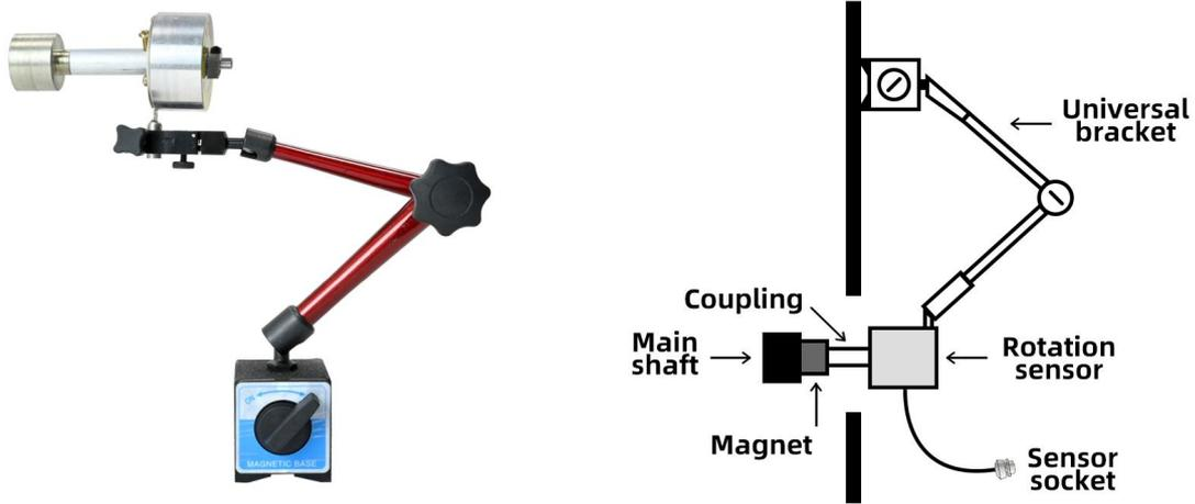
Outdoor SF6 circuit breakers whose speed is below 3.5m/S can be attracted to the main shaft with a magnet. If the speed exceeds this speed, it must be installed on the main shaft with a hard connection.
