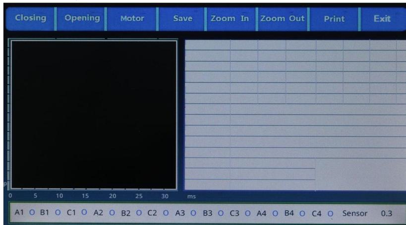
(1) **Closing test:** click this menu, closing voltage output, measuring closing time, bounce time and times, three-phase different period, speed and other parameters are displayed on the same screen, as shown below:
