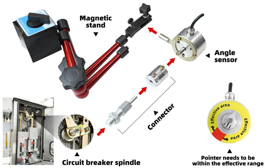
The arm of the SF6 circuit breaker has an angular displacement sensor connection port. Fix the U-shaped port in the screw hole correspondingly, and then fix the sensor with a universal joint. As shown below:
