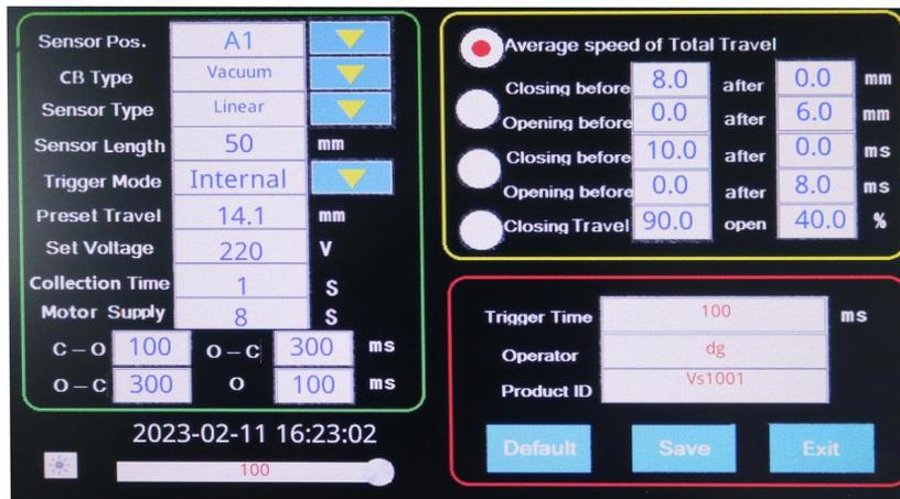
**(1) sensor location:** The default location of the sensor is A1 fracture, according to the actual situation of the sensor installation to set, such as accident speed travel, do not need to set.
