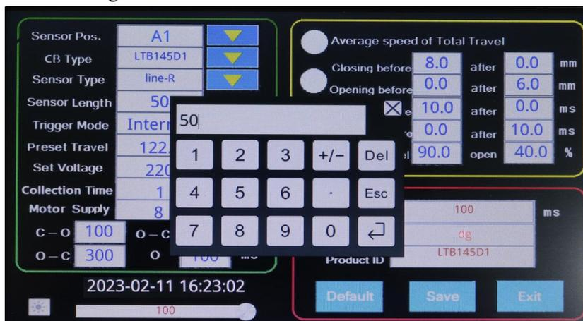
(5) **trigger mode:** trigger mode has inside trigger, outside trigger, from trigger (also known as manual trigger) three ways.
