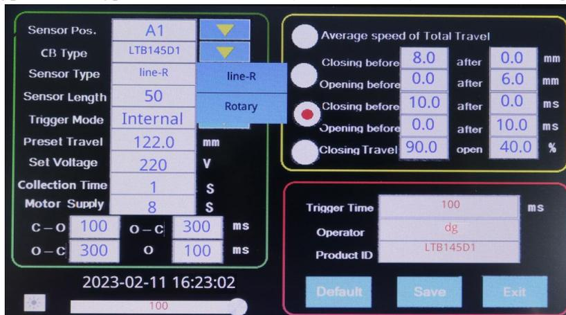
(4) **sensor length:** if the length of the linear sensor is 50mm, in addition, set 50, if it is 300 of the linear sensor will be set 300. According to the length of the sensor used for setting, the instrument adaptive calculation. Click the number, the keyboard pops up, Enter the correct number, and press Enter to confirm, as shown in the figure below:
