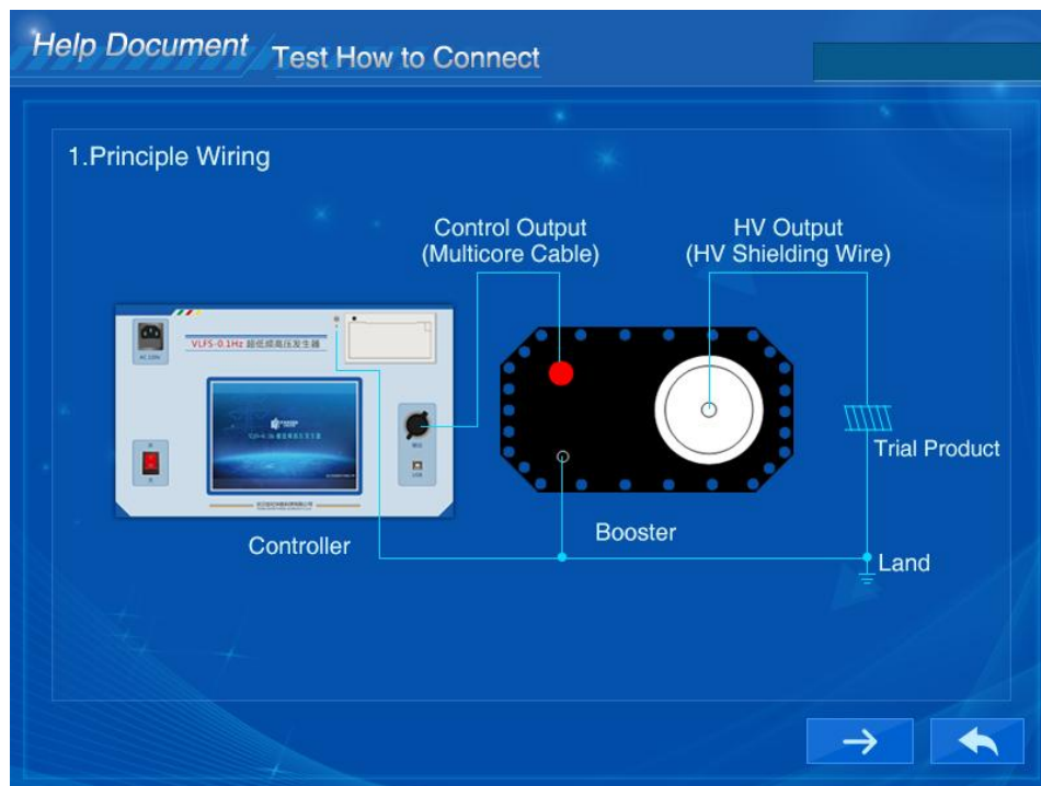
Figure 4 Schematic Diagram of Wiring
